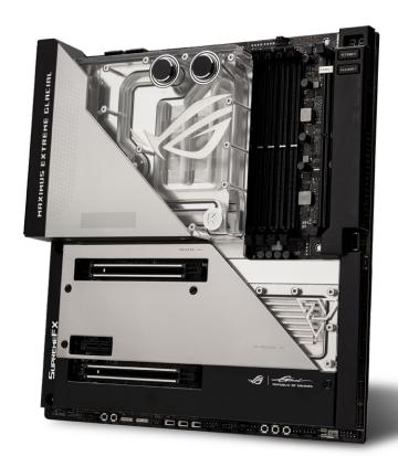
Making this happen by using a single piece of copper or standard milling was not possible. So, the following question was asked - why wouldn't we simply use the brazing process to join the top and bottom water block using copper tubes?
