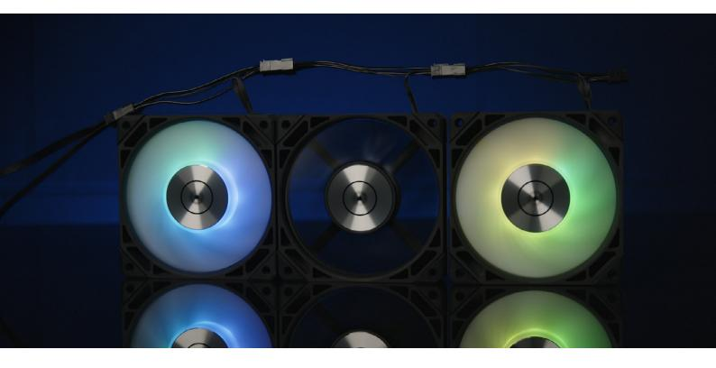
Each cable fits the length of a fan and has both male and female connectors. Every fan or device has all 8 of its pins connected in series, regardless of whether that product uses them or not, so a sequence of D-RGB lighting is not interrupted by a non-D-RGB fan.
