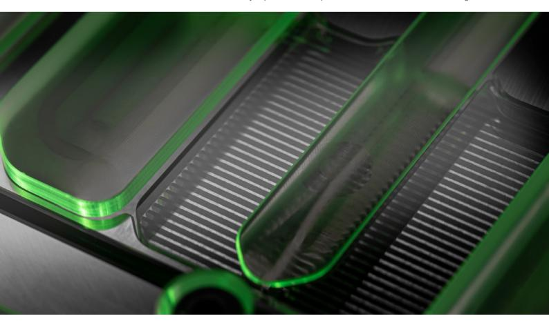
The jet plate is an integral part of the cooling engine, increasing the flow velocity through the fins and providing some obstruction to crudely distribute the flow, and it could not be removed entirely.
