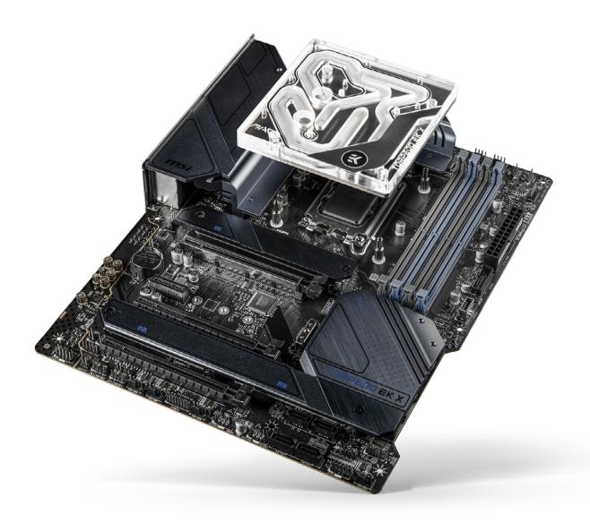
Here's how an Opti-socket works. The hybrid monoblock is normally mounted to cool the CPU. Additionally, there is a flat spot on the stock motherboard heatsink, right above the VRMs. Using thermal pads, the monoblock also makes contact with the already installed VRM heatsink. This design is simple and cost-effective but still allows us to utilize our latest Velocity Two cooling engine and, although indirectly, water-cool the CPU power delivery.
