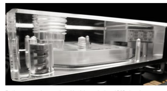
Furthermore, on the secondary side of the motherboard PCB, there is a height restriction preventing any significant protrusions. To package a coil spring, it was apparent that it had to be on the primary side; a thumb nut on the back could then pull on a screw to tension the spring.
