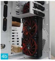
next to the motherboard, where there is enough space to fasten it on. The pump will fit nicely in the 5.25-inch drive bay. Important Note: Take care to not over-fasten the fans, it as you might accidentally puncture the radiator. Radiators often come with its own set of fasteners or screws, usually at the right length, but check them anyway. Most leaks in a water cooling setup are caused by negligence.
