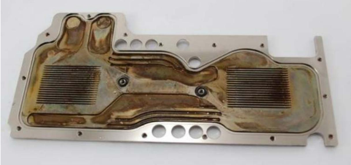
The stains/deposit on the nickel plated surface were clearly thick and ugly.
