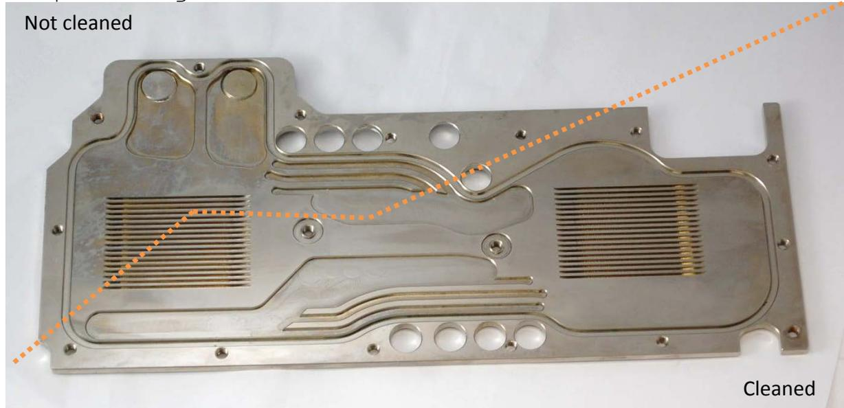
The block was easy to clean with a paper towel, and the original surface gloss was restored. No staining or discoloration remained after wiping.
