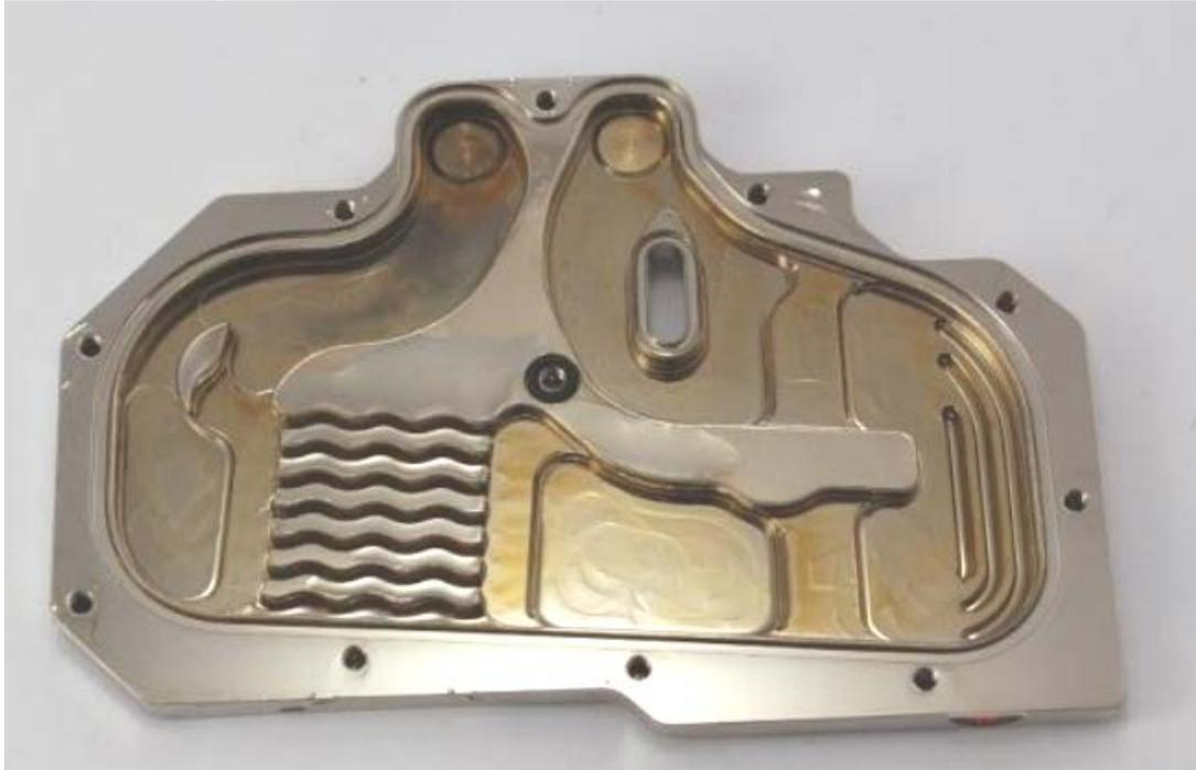
The discoloration/deposit on the nickel plated surface was not previously found in only distilled water systems. The discoloration/staining is very likely because of the high discoloration/staining of the EN block in the same loop, although much less intense. A standalone system has already been set up to exclude any influences from EN blocks on the nickel plated block.
