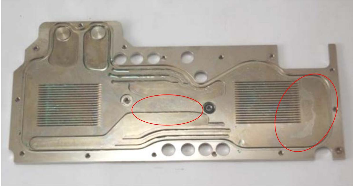
On the surface, only minor stains/discoloration can be seen caused by the drying layer of coolant. The slight blue cast that can be seen is due to the Blue Coolant.
