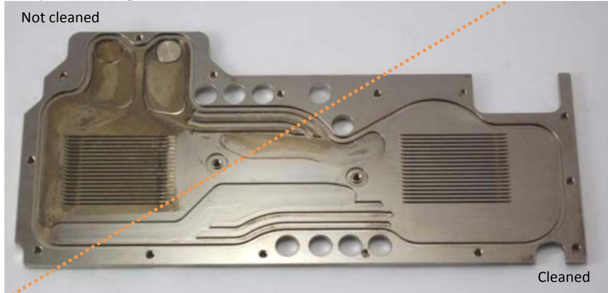
Cleaning was made by polishing paste and was pretty easy. Using a paper towel alone was not sufficient to clean the surface.
