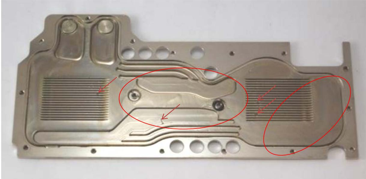
No excessive dirt/discoloration was found on the surface. However, we have found traces of gunking which appears to be plasticizer from the tubing (see red arrows).
