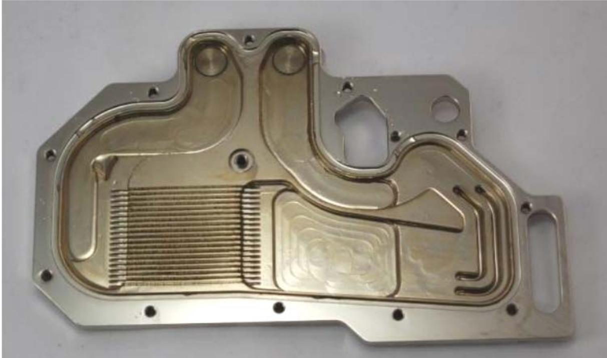
The discoloration/staining is very likely because of the high discoloration/staining of the EN block in the same loop.
