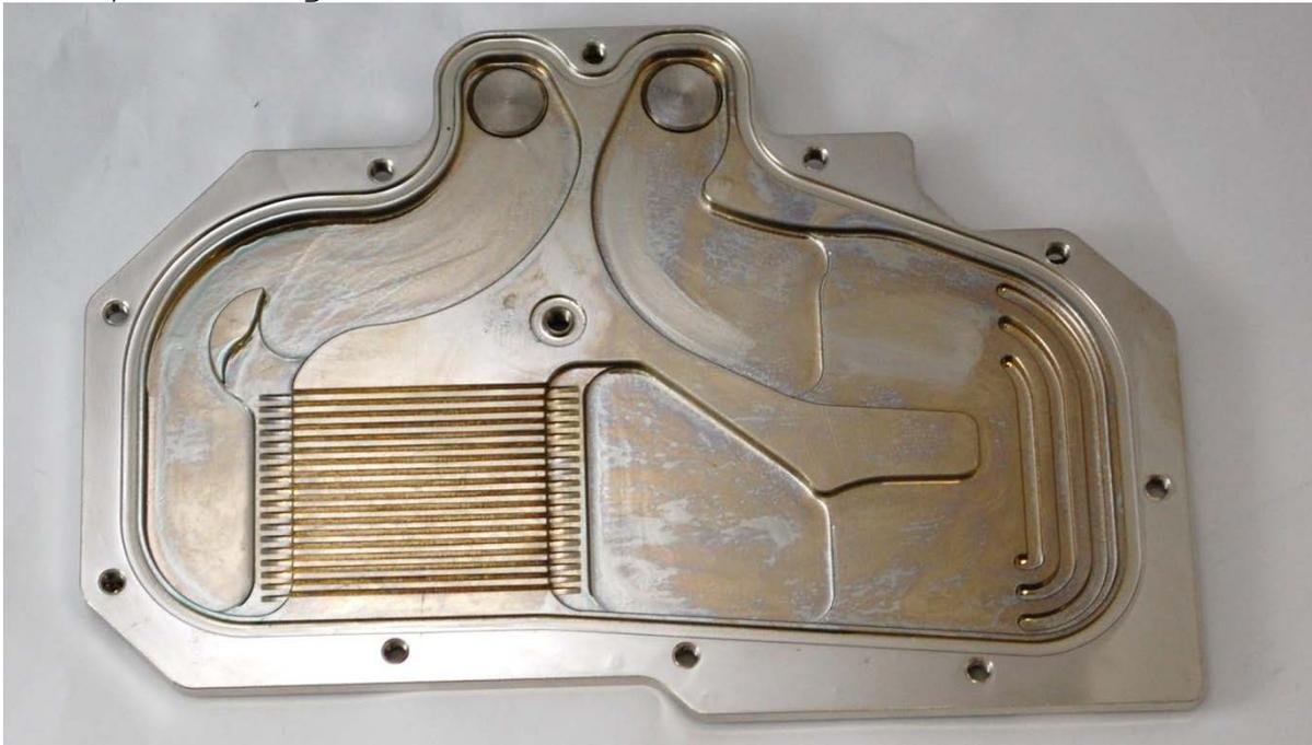
The dirt on the surface on the nickel plating was mainly dried coolant.
