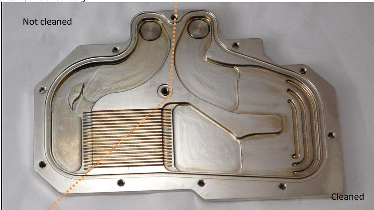
The block was easily cleaned with a paper towel, and the original surface gloss was restored. No staining or discoloration remained after wiping.
