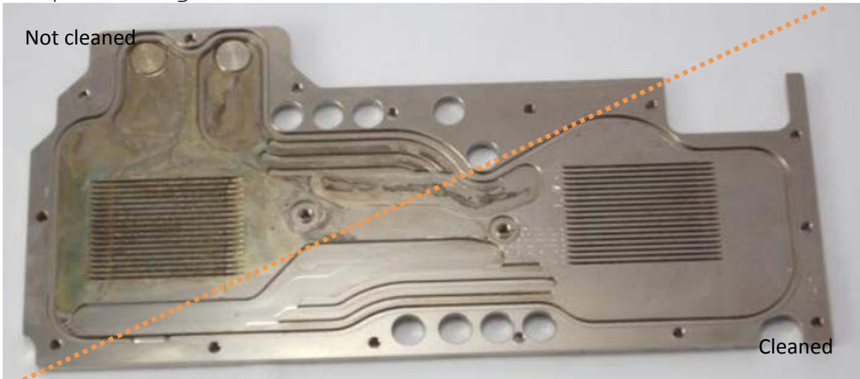
The degree of staining itself was lower when compared to that observed in the distilled water only loop. Cleaning was uncomplicated using the polishing paste, however using a paper towel alone was not sufficient to clean the surface.
