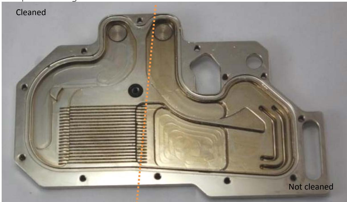
Cleaning with polishing paste needed little effort. Using a paper towel alone was not sufficient to clean the surface.
