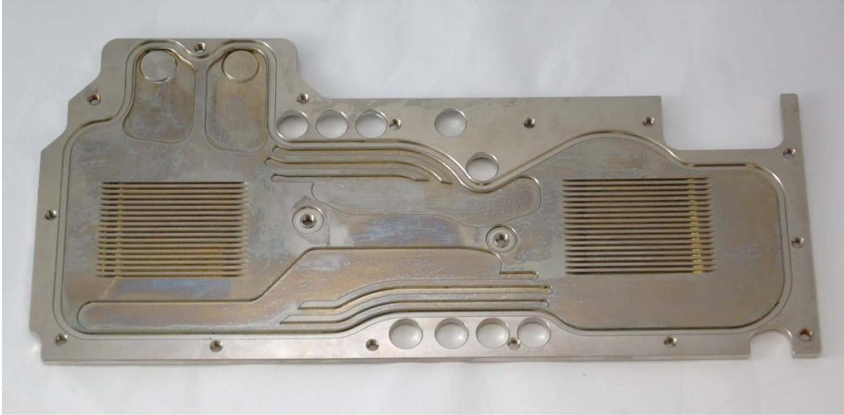
Only minor stain/discoloration can be seen on the surface, caused by the drying layer of coolant.
