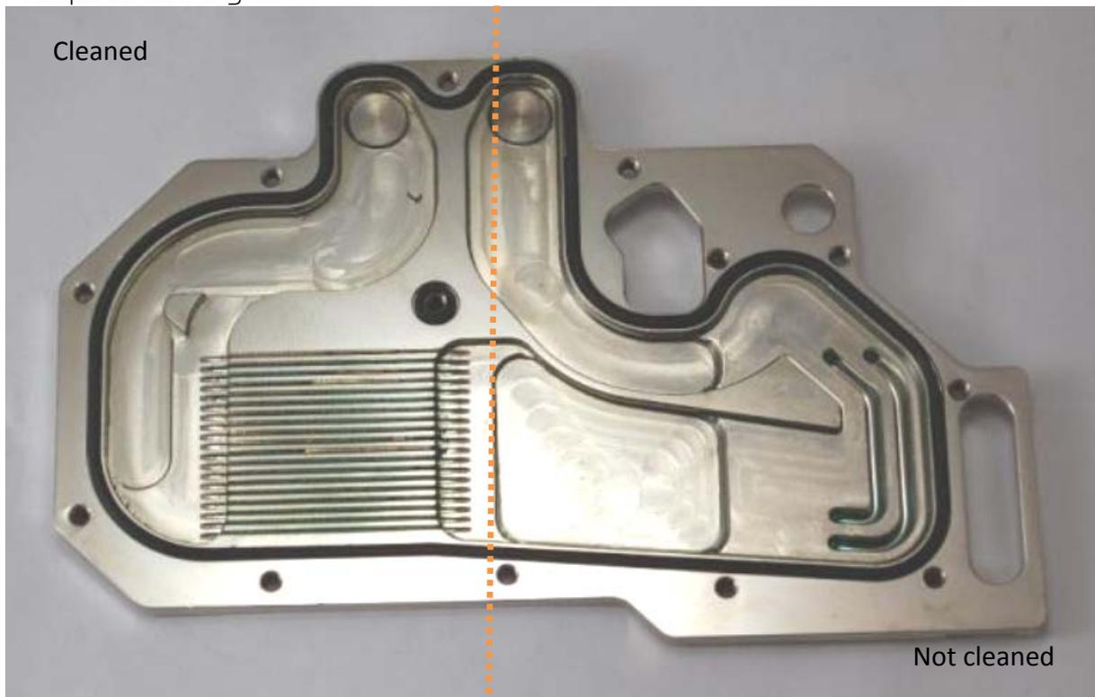
The areas where Ekoolant remained were easily wiped by a paper towel. No staining or discoloration remained after wiping.
