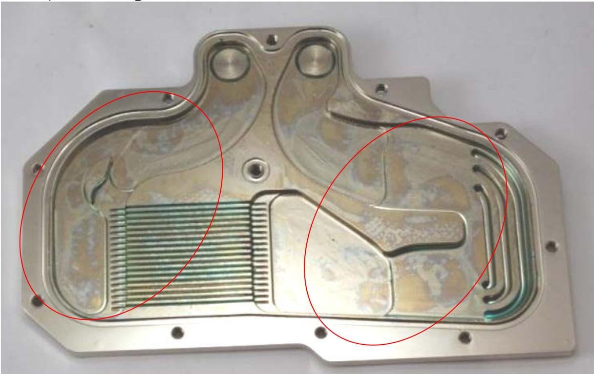
After opening the block, only a layer of drying coolant was left on the surface. The blue of the coolant is showing in the recessed areas where more of the blue coolant remained.
