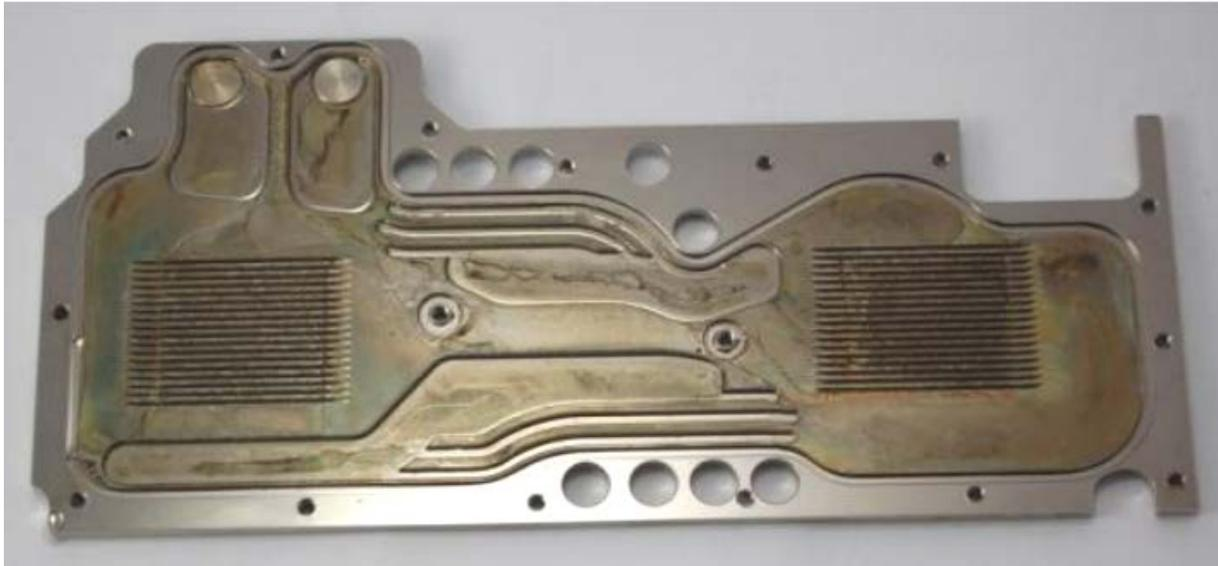
Before cleaning, the surface had similar but less intense discoloration/deposit compared to that observed in the distilled water only loop.
