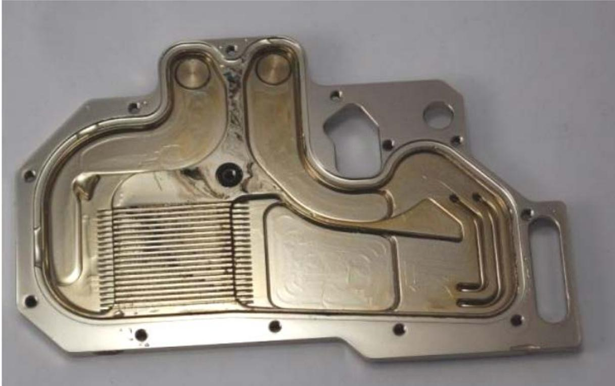
The block was cleaned using the polishing paste, as a paper towel alone was not sufficient to clean the surface. The result was as expected. There were already signs of possible corrosion at the those places where water flow is minimal – between the top and nickel plated base. The discoloration/staining is very likely because of the high discoloration /staining of the EN block in the same loop.
