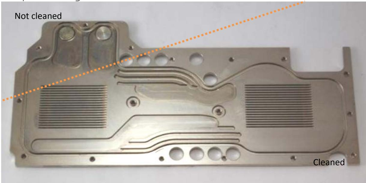
Cleaning the block was easy, although less so than in the loops where Ekoolant was used.
