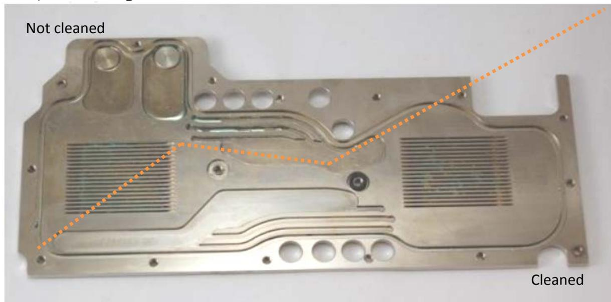
The internal channels of the block where Ekoolant was flowing were easily wiped by a paper towel. Discoloration is minimal.
