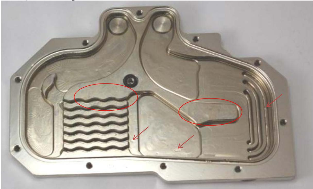
There was no excessive staining/dirt deposits found. However, we have found traces of gunking which appears to be plasticizer from the tubing.
