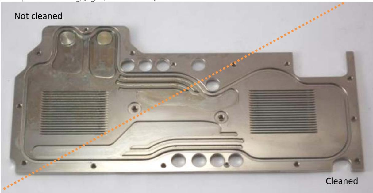
The area where we used Ekoolant was easily cleaned by wiping with a paper towel. Discoloration was minimal and is likely to have been caused by glycol.
