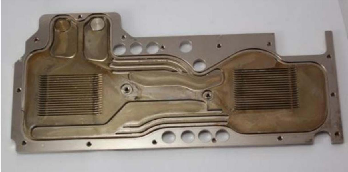
Before cleaning, the surface had similar discoloration/deposit when compared to the loop using distilled water only and the loop with Copper Sulphate based biocide.
