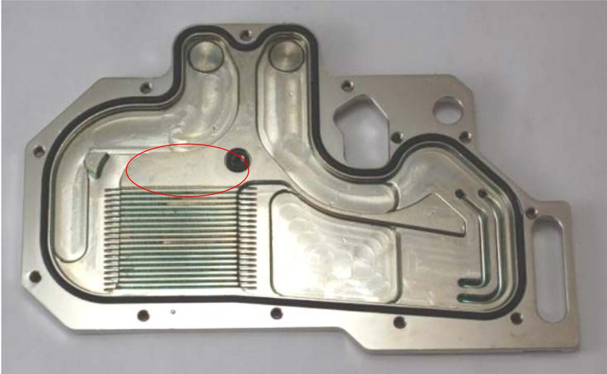
On the Galvanic nickel plated block used in the loop with Ekoolant, only minor staining/discoloration was detected.
