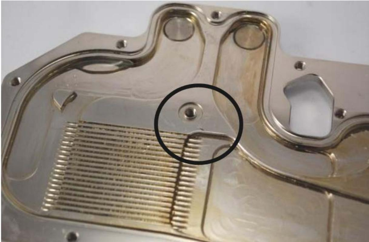
After cleaning the corrosion of the nickel plating was confirmed. The cleaning of the other surface was relatively easy.
