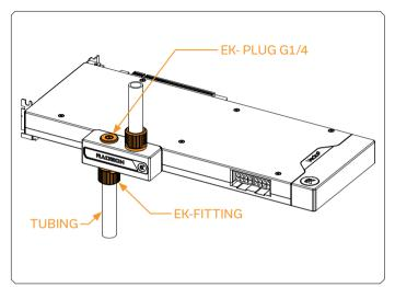
Screw in two (2) G1/4 threaded male fittings. Attach the liquid cooling tubes and connect the water block to the cooling loop.
