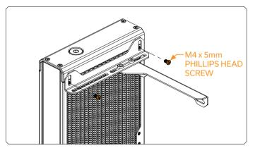
EK-Loop Angled Bracket - 140/120 mm can be mounted onto the 140 mm format radiator using the M4 x 5 mm Phillips head radiator mounting screws (as shown in the picture). There is no need for additional nuts, just tighten the screws evenly and do not use excessive force
