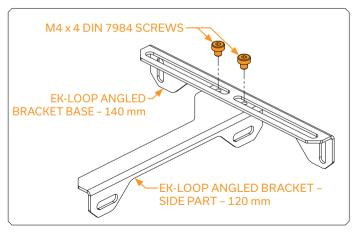
For the assembly of the EK-Loop Angled Bracket – 140/120 mm, use M4 x 4 DIN 7984 screws (as shown in the picture). Side parts already have threaded holes, so there is no need for additional washers and nuts.
