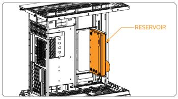
After securing the EK-Loop Angled Bracket – 140/120 mm into the chassis, you can attach the FLT reservoir. (See chapter: **Attaching the Reservoir to the EK-Loop Angled Bracket**)
