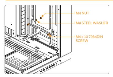
EK-Loop Angled Bracket - 140/120 mm can be mount directly into the case when there is a place for a 140 mm fan.
