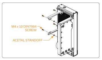
Carefully position the 120 format FLT reservoir onto the EK-Loop angled bracket and secure it with the enclosed M4 x 10 DIN 7984 screws and acetal standoffs (as shown in the picture). While tightening the screws, do not use excessive force. Make sure that all four (4) screws and standoffs are adequately secured!
