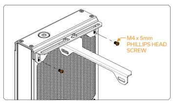
EK-Loop Angled Bracket - 140/140mm can be mounted onto the 140mm format radiator using the M4 x 5mm Phillips head radiator mounting screws (as shown in the picture). There is no need for additional nuts, just tighten the screws evenly and do not use excessive force
