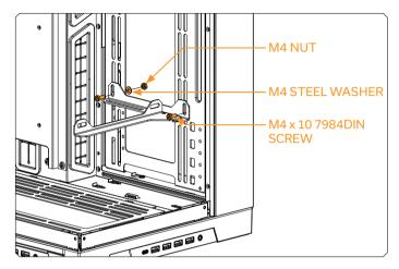
EK-Loop Angled Bracket - 140/140mm can be mount directly into the case when there is a place for a 140mm fan.
