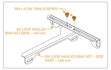
For the assembly of the EK-Loop Angled Bracket – 140/140 mm, use M4 x 4 DIN 7984 screws (as shown in the picture). Side parts already have threaded holes, so there is no need for additional washers and nuts.
