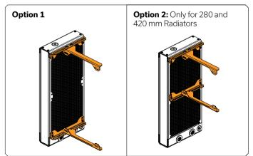
You can mount the bracket on each side of the radiator. On 280 and 420 mm radiators, the bracket can also be attached to the middle holes.
