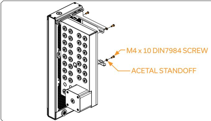
Carefully position the 140 format reservoir onto the EK-Loop angled bracket and secure it with the enclosed M4 X 10 DIN 7984 screws and acetal standoffs (as shown in the picture). While tightening the screws, do not use excessive force. Make sure that all four (4) screws and standoffs are adequately secured!
