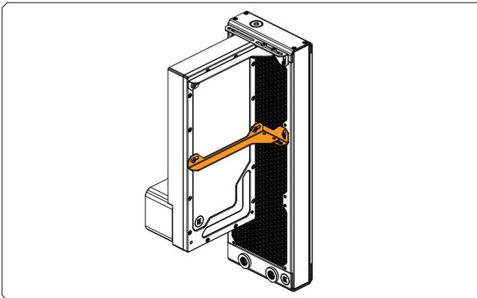
**When using the holes in the middle, it is no longer possible to move the FLT reservoirs from or toward the radiator!**
