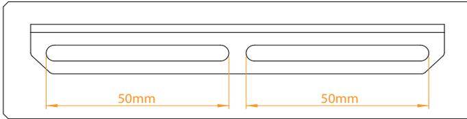
EK-Loop Angled Bracket base piece has four slot holes that allow adjustability. Larger slot holes will enable adjusting of the bracket's position (50 mm on each side). Side pieces can be screwed into the base through one of the slots or both of them.
