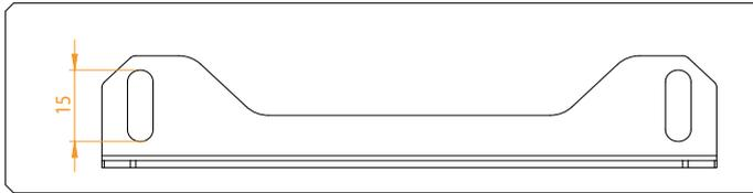
Smaller slot holes on the side allow for adjusting the position of the bracket on the radiator.
