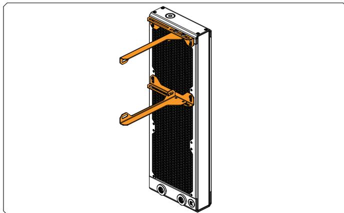
You can mount the bracket on each side of the radiator. On 240, 360 and 480 mm radiators, the bracket can also be attached to the middle holes.
