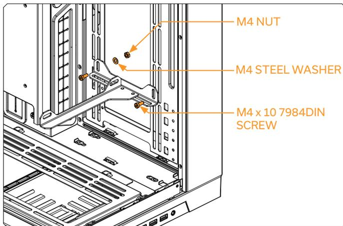
EK-Loop Angled Bracket - 120/140 mm can be mount directly into the case when there is a place for a 140 mm fan.
