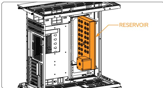
After securing the EK-Loop Angled Bracket - 120/140mm into the chassis, you can attach the reservoir. (See chapter: **Attaching the Reservoir to the EK-Loop Angled Bracket**)
