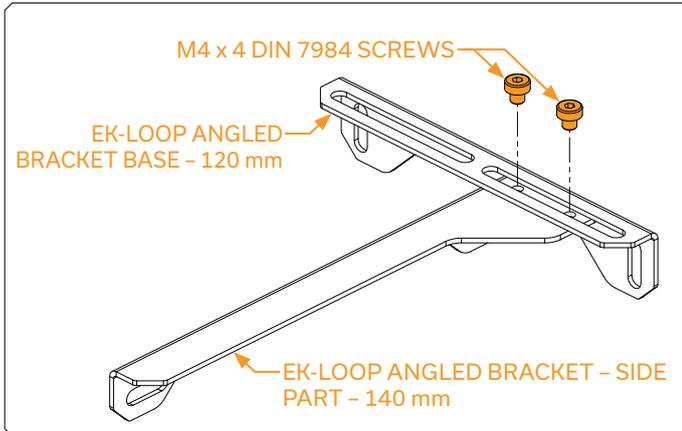
For the assembly of the EK-Loop Angled Bracket - 120/140 mm, use M4 x 4 DIN 7984 screws (as shown in the picture). Side parts already have threaded holes, so there is no need for additional washers and nuts.
