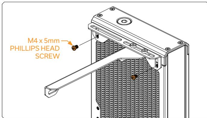
EK-Loop Angled Bracket - 120/140 mm can be mounted onto the 120 mm format radiator using the M4 x 5 mm Phillips head radiator mounting screws (as shown in the picture). There is no need for additional nuts, just tighten the screws evenly and do not use excessive force.
