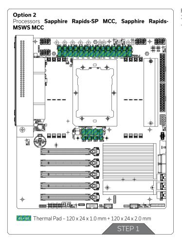
Replacement thermal pads: **Option 2** 3x Thermal PAD G 1.0 mm - (120 x 24 mm) EAN: 3830046996770 + 3x Thermal PAD G 2.0 mm - (120 x 24 mm) EAN: 3830046996794
