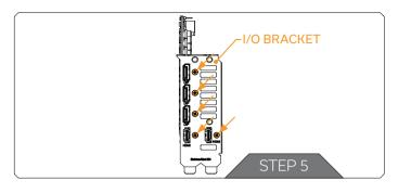
Lastly, unscrew five (5) Screws and detach the I/O Bracket (using Phillips head screwdriver).
