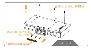
Place five (5) M3 x 10 AX1 screws into the water block standoffs and tighten them using a Philips head screwdriver (as shown in the image). After attaching the AX1 Screws, three (3) terminal screws M4 x 20 DIN7984 need to be attached using Allen Key 2.5 mm. The terminal badge can be reused, after securing the terminal screws.
