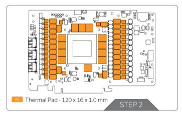
Once cut to the size, Thermal Pads should be placed on the PCB, as shown in the picture:
