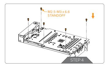
After securing the GPU PCB, position the five (5) M2.5-M3  $\times$  6.6 standoffs. Tighten it with the provided tool (EK-Plug out Spludger Tool).
