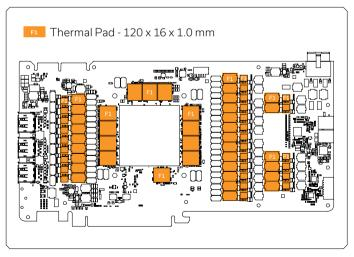
Your EK-Quantum Vector<sup>2</sup> Strix/TUF RTX 3090 Ti D-RGB block comes with Thermal Pads that have to be cut into smaller pieces to cover all the VRM components. EK made sure to provide you with more than an adequate quantity of Thermal Pads to complete this Step.
