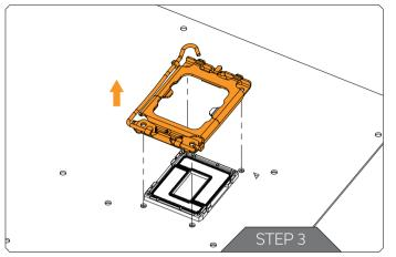
Remove the stock mounting mechanism from the motherboard to remove the stock motherboard backplate.
