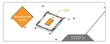
**Cleaning the CPU:** Wipe the DIE clean using a non-abrasive cloth or Q-tip.
