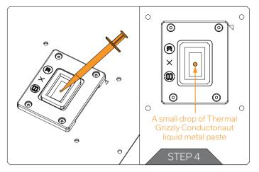
Apply a small drop of Thermal Grizzly Conductonaut liquid metal paste and spread it evenly over the DIE with cotton swabs that are included in the bag. Use the provided needle accessory that is included in the bag. Don't press the syringe too hard!
