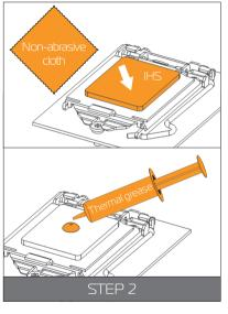
**Cleaning the CPU:** Wipe the CPU's contact surface (by using non-abrasive cloth or Q-tip, as shown on sample photo).
