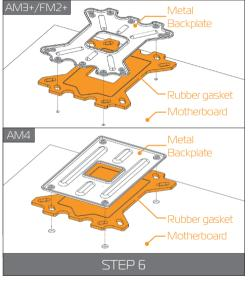
Install backplate rubber gasket and place metal backplate for AMD® socket to the back of your motherboard RIBBED SIDE UP! (facing away from the motherboard) Align the holes on the motherboard with holes on rubber gasket and backplate.
