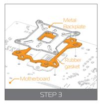
Install backplate rubber gasket and place metal backplate for Intel® LGA-115x socket to the back of your motherboard RIBBED SIDE UP! (facing away from the motherboard) Align the holes on the motherboard with holes on rubber gasket and backplate.
