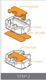
Unscrew the four M4 screws in counter-clockwise direction from the bottom of the water block using enclosed 2,5mm Allen key to release the assembly, consisting of water block top, the insert, insert pin and jet plate. Upon replacing the insert and/or jet plate please re-assemble the water block as shown on the photo in STEP 1 and STEP 2. Pay special attention to the insert orientation relative to the copper base and water block top!
