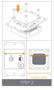
Replace the Intel® factory installed mounting plate with AMD® one. You will feel the mounting plate locking into the position when placed correctly on to the top.
