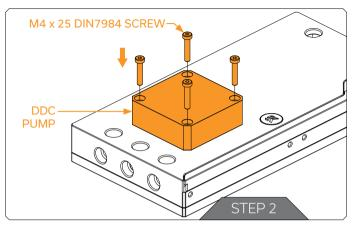
Carefully attach the DDC pump and make sure that gasket ( $46 \times 2.5$ ) is placed correctly. Sealing gasket is included in additional bag. Secure the pump with four (4) M4 x 25 7984DIN screws. Tighten the screws using enclosed 2.5 mm Allen Key.
