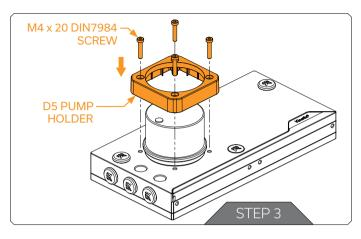
Carefully attach the D5 Pump and Pump Holder(as shown in the photo). After that, secure all the parts together with M4  $\times$  20 DIN 7984 Screws. Tighten the screws using the enclosed 2.5 mm Allen Key.
