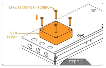
Carefully attach the VTX pump and make sure that the gasket (46 x 2.5) is placed correctly. A sealing gasket is included in the additional bag. Secure the pump using the four M4 x 35 7984DIN screws provided with the VTX pump. Tighten the screws using the enclosed 2.5 mm Allen Key.
