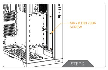
To secure the reservoir, use four (4) M4x8 DIN7984 screws using  $2.5\,$  mm allen key.
