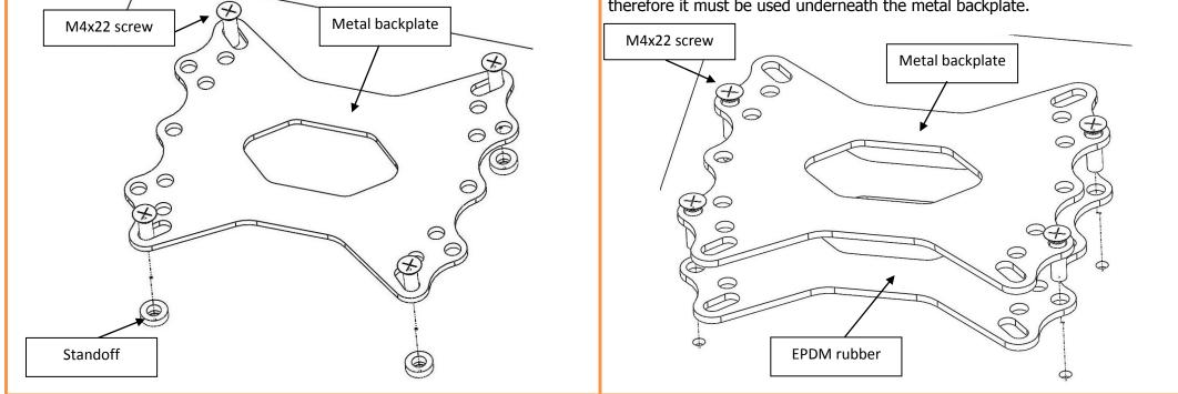
When using motherboard with Intel LGA-1155/1156 socket, insert screws at positions as shown bellow. Standoffs are used to prevent possible overtightening of screws and causing potentional damage to PCB. EPDM rubber must be used in order to prevent socket latch backplate damage.
