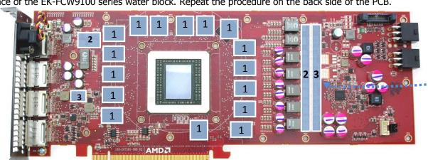
2. PLACING BLOCK TO GRAPHIC CARD. Carefully position the water block with preinstalled 2.5mm standoffs on to the graphics card. During this process please make sure you align mounting holes on PCB with holes on the water block. Also pay attention not to use too much force by pressing block down to PCB. Chip dies are prone to cracking.
