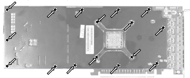
2. CLEANING THE PCB. Carefully detach the original stock cooler after removing **all** screws securing it to the board. Wipe off the remains (by using non–abrasive cloth or *qtip*, as shown on sample photo) of the original thermal compound until the components and circuit board are completely clean. EKWB recommends the use of denatured alcohol for removing TIM leftovers.
