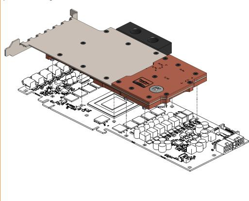
3. ATTACHING BLOCK TO GRAPHIC CARD. By using Philips screwdriver screw in enclosed M3x4 DIN7985 screws, afterwards use enclosed Allen key 2mm to tighten the remaining M3x8 DIN7991 screws in order to secure the factory provided backplate. Use plastic washers and M3 nuts to secure the three screws near the power connectors as shown on picture below. EKWB recommends users. Always use a plastic washer under each DIN7985 type screw!
