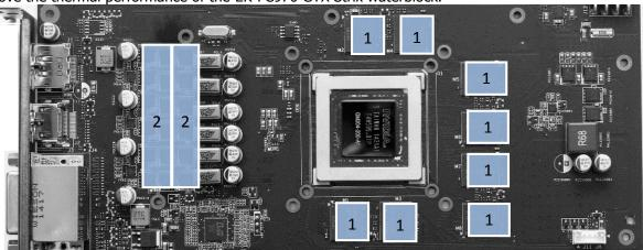
2. PLACING THE BLOCK ON TO THE GRAPHICS CARD. Carefully position the water block with preinstalled standoffs on to the graphics card. During this process please make sure you align mounting holes on the PCB with holes on the water block (same applies for other tops). Also pay attention not to use too much force by pressing the block down to the PCB. Chip dies are prone to cracking.
