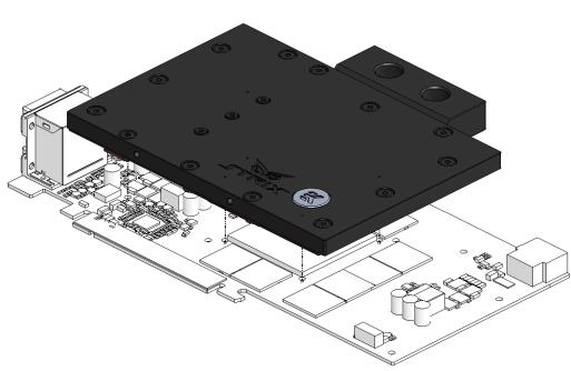
3. ATTACHING THE BLOCK TO THE GRAPHIC CARD. Use a Philips screwdriver with the enclosed M3x4 DIN 7985 screws. EKWB recommends users to start tightening the screws around the GPU core and continue outwards.
