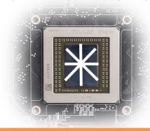
4. CUTTING THERMAL PADS. Your block comes with thermal pads, some of which are already pre-cut. Others have to be cut to smaller chunks in order to cover all the VRM components such as MOSFETs and drivers. PLEASE REMOVE THE PROTECTIVE FOIL FROM BOTH SIDES OF THE THERMAL PADS PRIOR TO INSTALLATION.
