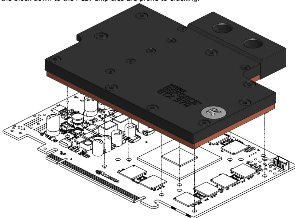
3. **ATTACHING THE BLOCK TO THE GRAPHIC CARD.** Use a Philips screwdriver screw with the enclosed M3x4 DIN 7985 screws. EKWB recommends users to start tightening the screws around the GPU core and continue outwards. Always use a plastic washer under each and every screw!
