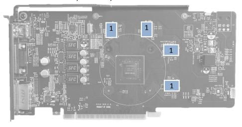
2. PLACING THE BLOCK TO THE GRAPHICS CARD. Carefully position the water block with preinstalled 2.1 mm standoffs on to the graphics card. During this process please make sure you align mounting holes on the PCB with holes on the water block. Also pay attention not to use too much force by pressing block down to PCB. Chip dies are prone to cracking.
