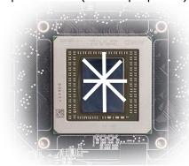
4. CUTTING THERMAL PADS. Your block comes with thermal pads, some of which are already pre-cut. Others have to be cut to smaller chunks in order to cover all the VRM components such as MOSFETs and drivers. PLEASE REMOVE THE PROTECTIVE FOIL FROM BOTH SIDES OF THE THERMAL 100
