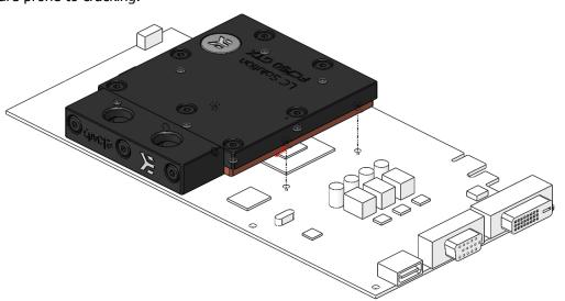
3. ATTACHING BLOCK TO THE GRAPHIC CARD. Use a Philips screwdriver screw in enclosed M2.5 x4 DIN 7985 screws. EKWB recommends users to start tightening the screws around the GPU core and continue outwards.
