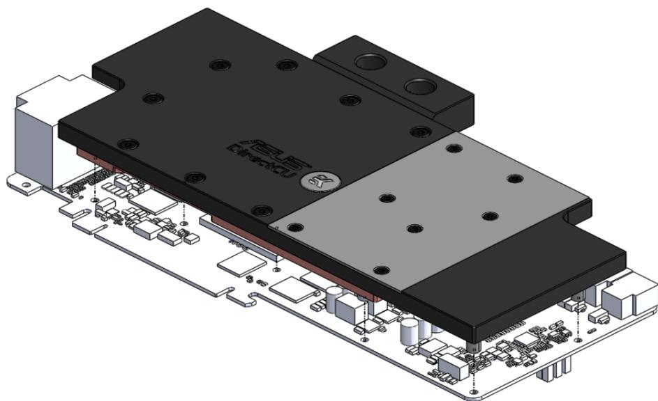
3. **ATTACHING THE BLOCK TO THE GRAPHIC CARD.** Use a Philips screwdriver screw with the enclosed M3x4 DIN 7985 screws. EKWB recommends users to start tightening the screws around the GPU core and continue outwards.
