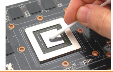
3. APPLYING THERMAL COMPOUND. Wipe off the remains (by using non–abrasive cloth or *q-tip*) of the original thermal compound until the components and circuit board are completely clean. Apply thermal compound: lightly coat AMD GPU chip with enclosed EK-TIM Ectotherm thermal grease. EKWB recommends to apply thermal grease in cross form for best performance (see sample picture).
