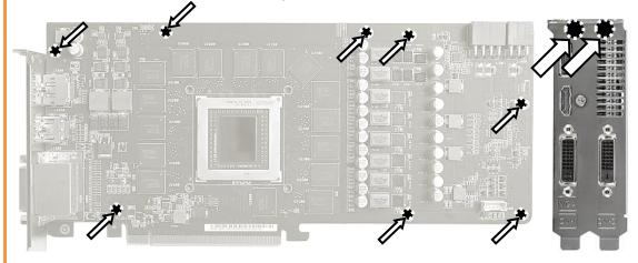
after removing **all** screws securing it to the board. Wipe off the remains (by using non-abrasive cloth or *qtip*, as shown on sample photo) of the original thermal compound until the components and circuit board are completely clean. EKWB recommends the use of denatured alcohol for removing TIM leftovers.
