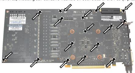
2. CLEANING THE PCB. Carefully detach the original stock cooler after removing **all** screws securing it to the board. Wipe off the remains (by using non–abrasive cloth or *q-tip*, as shown on sample photo) of the original thermal compound until the components and circuit board are completely clean. EKWB recommends the use of denatured alcohol for removing TIM leftovers.
