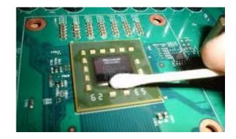
3. APPLYING THERMAL COMPOUND. Wipe off the remains (by using non–abrasive cloth or *q-tip*) of the original thermal compound until the components and circuit board are completely clean. Apply thermal compound: lightly coat *NVIDIA* GPU chip with enclosed EK-TIM Ectotherm thermal grease. EKWB recommends to apply thermal grease in cross form for best performance (see sample picture).
