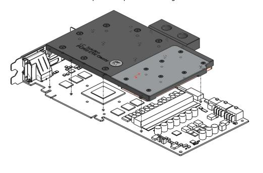
3. ATTACHING THE BLOCK TO THE GRAPHIC CARD. Use a Philips screwdriver screw with the enclosed M3x4 DIN 7985 screws. EKWB recommends users to start tightening the screws around the GPU core and continue outwards. Always use a plastic washer under each and every screw!
