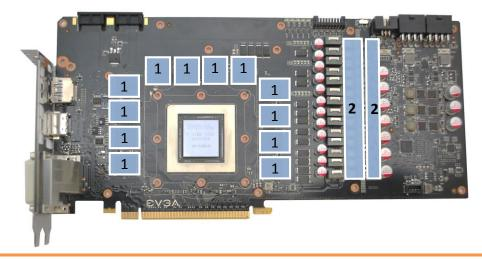
2. PLACING THE BLOCK ON TO THE GRAPHICS CARD. Carefully position the water block with preinstalled 2.5 mm standoffs on to the graphics card. During this process please make sure you align mounting holes on the PCB with holes on the water block (same applies for other tops). Also pay attention not to use too much force by pressing the block down to the PCB. Chip dies are prone to cracking.
