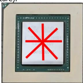
4. **CUTTING THERMAL PADS.** Your block comes with thermal pads, some of which are already pre-cut. Others have to be cut to smaller chunks in order to cover all the VRM components such as MOSFETs and drivers. PLEASE REMOVE THE PROTECTIVE FOIL FROM BOTH SIDES OF THE THERMAL PADS PRIOR TO INSTALLATION. Replacement thermal pads: Thermal Pad D – 0.5mm (RAM 8x), Thermal Pad A – 0.5mm.
