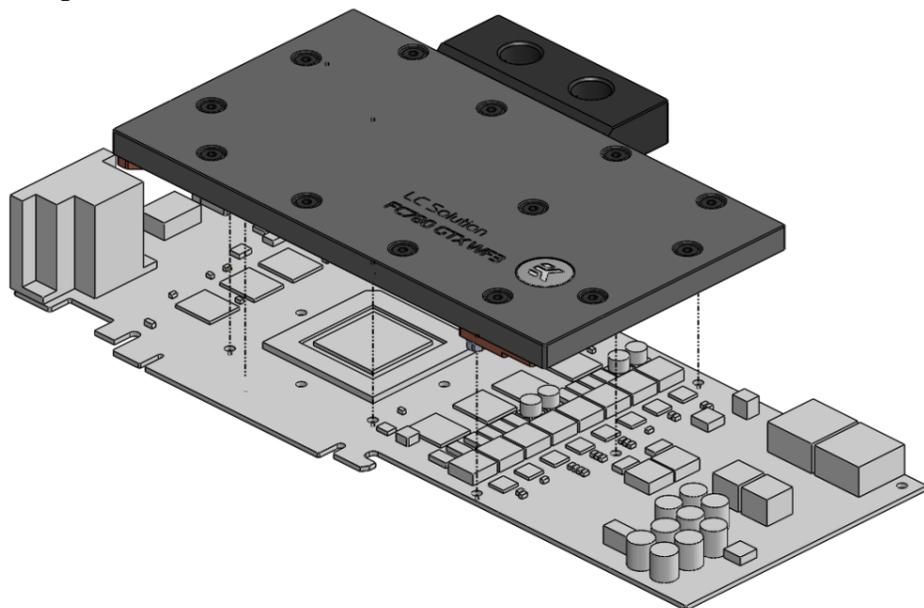
3. **ATTACHING BLOCK TO GRAPHIC CARD.** By using Philips screwdriver screw in enclosed M3x4 DIN7985 screws. EKWB recommends users to start tightening the screws around the GPU core and continue outwards. Always use a plastic washer under each and every screw!
