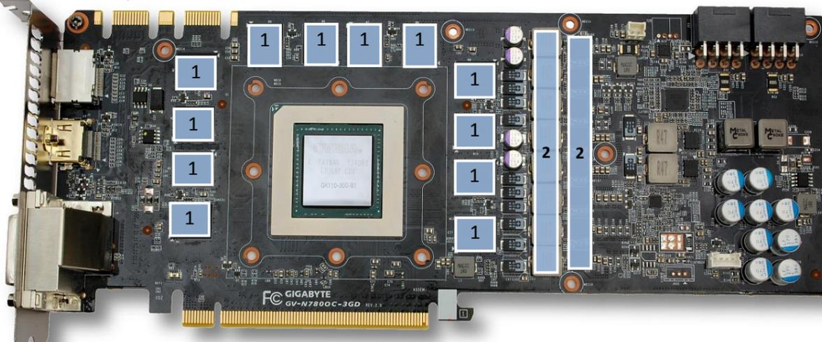
2. **PLACING BLOCK TO GRAPHIC CARD.** Carefully position the water block with preinstalled 2.5 mm standoffs on to the graphics card. During this process please make sure you align mounting holes on PCB with holes on the water block. Also pay attention not to use too much force by pressing block down to PCB. Chip dies are prone to cracking.
