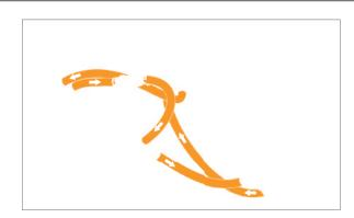
When changing the original EK ZMT tubing for transparent tubing (Primo-Chill Primo-Flex $^{\text{TM}}$  Advanced LRT $^{\text{TM}}$  9,5 mm (3/8") / 15,9 mm (5/8") - Crystal Clear tube) or equivalent it may happen that the coolant evaporates through the tubing walls due to PVC material being slightly porous.
