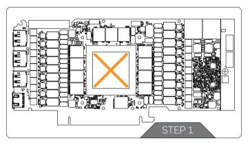
Apply the enclosed EK-TIM Ectotherm thermal grease (thermal compound) on the GPU heat spreader – IHS – as shown in the image. The layer of the thermal compound must be thin and evenly spread over the entire surface of the IHS.
