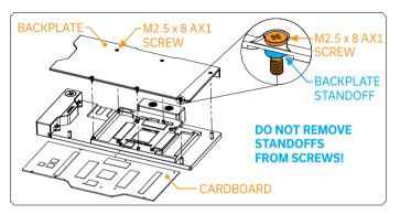
Unscrew six (6) Screws AX1 M2.5x8 as shown in the image. Remove the backplate together with six (6) Screws AX1 M2.5x8 and six (6) backplate standoffs. Standoffs must stay on Screws AX1 M2.5x8. Remove PCB cardboard. Do not remove standoffs from screws! In case the standoff detaches from screw, replace it with a spare one. When replacing the standoff make sure that you screw it onto AX1 M2.5x8 screw. Do not push the standoff onto the screw AX1 M2.5x8!
