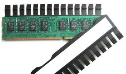
Carefully remove the factory installed heat spreaders using screwdriver, sharp blade or heat, depending on the type of assembly.
