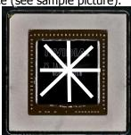
4. CUTTING THERMAL PADS. Your block comes with thermal pads, some of which are already pre-cut. Others have to be cut to smaller chunks in order to cover all the VRM components such as MOSFETs and drivers. PLEASE REMOVE THE PROTECTIVE FOIL FROM BOTH SIDES OF THE THERMAL PADS PRIOR TO INSTALLATION. Replacement thermal pads: Thermal Pad D – 0.5mm (RAM 8x), Thermal Pad B – 0.5mm (75x50mm)
