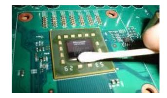
3. APPLYING THERMAL COMPOUND. Wipe off the remains (by using non–abrasive cloth or *qtip*) of the original thermal compound until the components and circuit board are completely clean. Apply thermal compound: lightly coat *NVIDIA* GPU chip with enclosed Arctic Cooling MX-2 ™ thermal grease. EKWB recommends to apply thermal grease in cross form for best performance (see sample picture).
