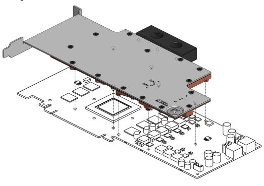
3. ATTACHING BLOCK TO GRAPHIC CARD. By using Philips screwdriver screw in enclosed M3x4 DIN7985 screws. EKWB recommends users to start tightening the screws around the GPU core and continue outwards. <u>Always use</u> a plastic washer under each and every screw!
