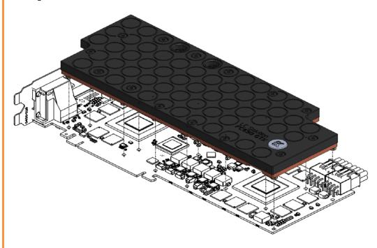
3. ATTACHING BLOCK TO GRAPHIC CARD. By using Philips screwdriver screw in enclosed M3x4 DIN7985 screws. EKWB recommends start screwing the screws around the GPU core using Philips head screwdriver and continue outwards. Always use a PVC washer under each and every screw!
