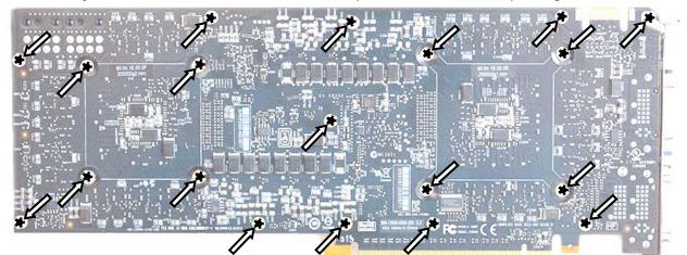
2. CLEANING THE PCB. Carefully detach the original stock cooler after removing all screws securing it to the board. Wipe off the remains (by using non-abrasive cloth or qtip, as shown on sample photo) of the original thermal compound until the components and circuit board are completely clean. EKWB recommends the use of denatured alcohol for removing TIM leftovers.
