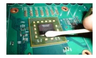
3. APPLYING THERMAL COMPOUND. Apply thermal compound: lightly coat both nVidia GPU chips as well as PLX bridge chip with for example Arctic Cooling MX-2 ™,MX-4 ™ or GELID GC-Extreme ™ thermal grease. EKWB recommends to apply thermal grease in cross form for best performance (see sample picture).
