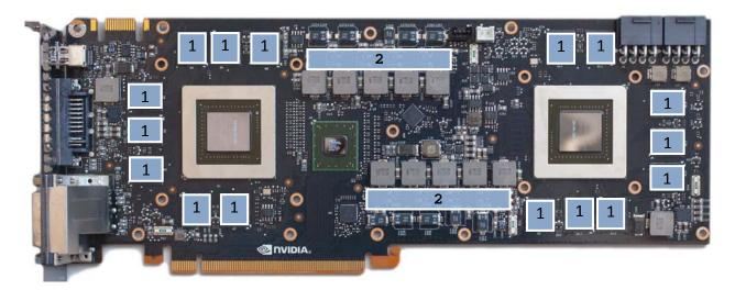
2. PLACING BLOCK TO GRAPHIC CARD. Carefully position the water block with preinstalled 2.5mm standoffs on to the graphics card. During this process please make sure you align mounting holes on PCB with holes on the water block. Also pay attention not to use too much force by pressing block down to PCB. Chip dies are prone to cracking.
