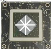
5. PLACING THERMAL PADS ON PCB. Place thermal pads on chips so that numbers on chips match size of thermal pads. Thermal pad number 1, 2 and 3 will have to be cut by user to match all small power regulation chips (EKWB made sure users have more than enough pads to cover all surfaces that need to be covered to make block fully function). You can also use small drop of thermal grease on chips to make thermal pads more adhesive.
