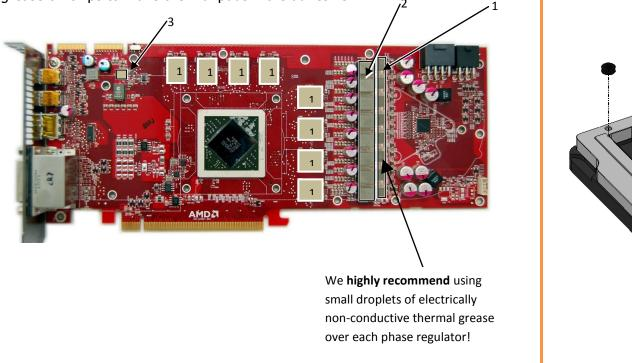
2. CLEANING THE PCB. Carefully detach the original heat sink after removing <u>all</u> fasteners securing it to the board and bracket. Wipe off the remains (by using nonabrasive cloth or Q-tip, as shown on sample photo) of the original thermal compound until the components and circuit board are completely clean. EKWB does not recommend using any liquids for removing paste.
