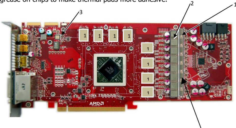
We highly recommend using small droplets of electrically non-conductive thermal grease over each phase regulator!
