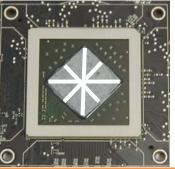
4. CUTTING THERMAL PADS. Your block comes with thermal pads, which have to be placed on chips (PLEASE REMOVE FOIL ON BOTH SIDES OF THERMAL PADS PRIOR TO INSTALLATION. WARNING: DIMENSION OF THE PADS BELLOW ARE SCALED.)
