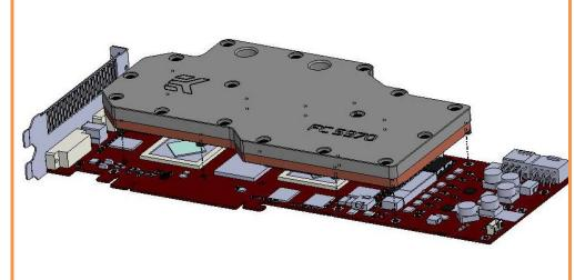
8. ATTACHING BLOCK TO GRAPHIC CARD. By using Philips screwdriver screw in enclosed M3x6 and M3x10 screws into the block. EKWB recommends start screwing the screws around the GPU core and continue outwards.
