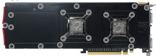
2. CLEANING THE PCB. Carefully detach the original backplate and stock cooler after removing <u>all</u> fasteners securing it to the board and bracket. Wipe off the remains (by using non-abrasive cloth or Q-tip, as shown on sample photo) of the original thermal compound until the components and circuit board are completely clean. EKWB does not recommend using any liquids for removing paste.
