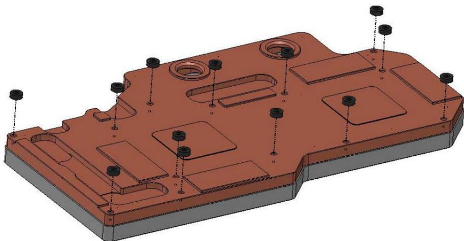
7. PLACING BLOCK TO GRAPHIC CARD. During this process please make sure you align holes on PCB with holes on block. Also pay attention not to use too much force by pressing block down to PCB. Chips are prone to cracking.
