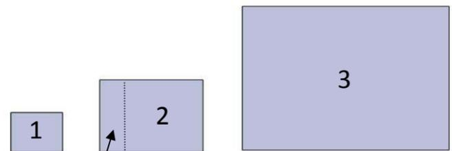
5. PLACING THERMAL PADS ON PCB. Place thermal pads on chips so that numbers on chips match size of thermal pads. Thermal pad number 2,3 will have to be cut by user to match all small chips (EKWB made sure users have more than enough pads to cover all surfaces that need to be covered to make block fully function). You can also use small drop of thermal grease on chips to make thermal pads more adhesive.
