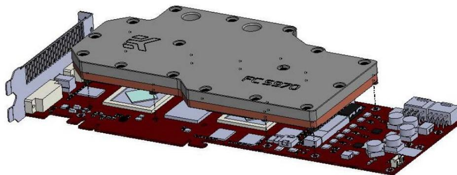
8. ATTACHING BLOCK TO GRAPHIC CARD. By using Philips screwdriver screw in enclosed M3x6 and M3x10 screws into the block. EKWB recommends start screwing the screws around the GPU core and continue outwards.
