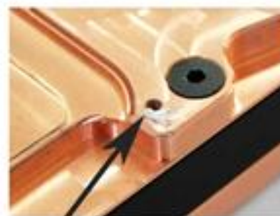
Apply little thermal grease near the threads in copper.
