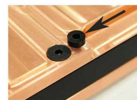
Then put the Stand-offs in center of the threads. Thermal grease helps that the stand-offs dont move while installing.
