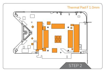
Once cut to size thermal pads should be applied to the PCB as shown in the image.
