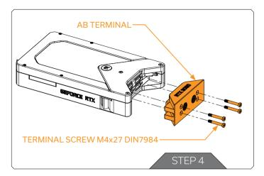
Set the Active backplate terminal in place with the preinstalled metal plate and secure it with four (4) M4x27 DIN7984 Screws. Tighten them evenly with the provided 2.5 mm Allen Key.
