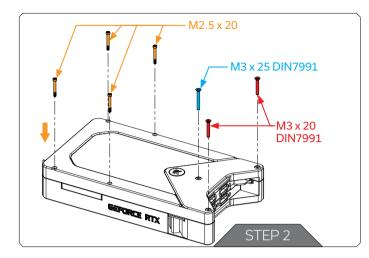
Place the active backplate on the PCB and make sure all holes are aligned. Position the screws in each of the seven (7) mounting holes (as shown in the image) and tighten them evenly with Allen Key 2 mm.
