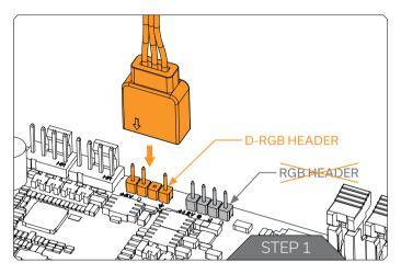
Plug the **3-pin connector** of the D-RGB LED strip to the **D-RGB HEADER** on the motherboard. The LED will work if the pin layout on the header is as follows: **+5V, Digital, Empty, Ground**.
