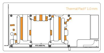
Your GPU water block comes with un-cuted thermal pads to cover all the VRM components, such as COILs, MOSFETs, and drivers. Please use 1,0mm thick thermal pads which should be placed on the water block, as illustrated below. EK made sure to provide you with more than an adequate quantity of thermal pads to complete this Step.
