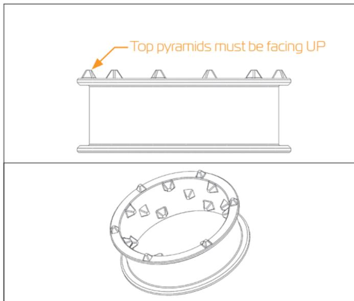
Additional Revo D5 Damper is enclosed. If pump vibrations are higher than expected additional Revo D5 Soft damper can be used. When replacing damper, take care that top pyramids are faced up as shown on picture below. In case of severe tilting of the computer chassis reservoir unit may fall out of the holder. Additional damper use is recommended in vertical reservoir unit mount
