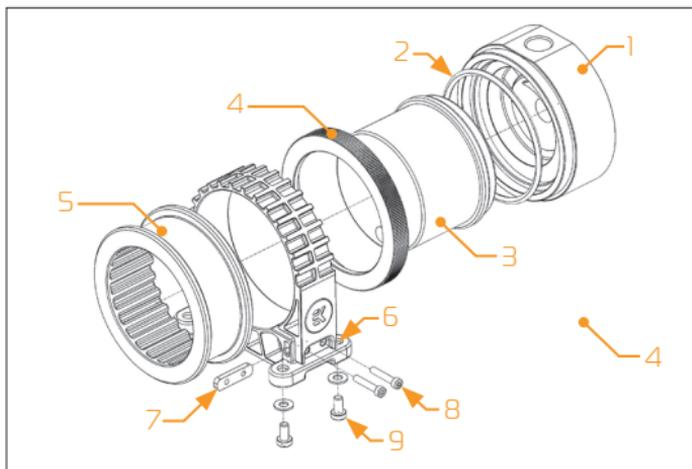
XTOP comes in two (2) port version. Pump Top has central inlet port and side OUTLET port (see picture above).
