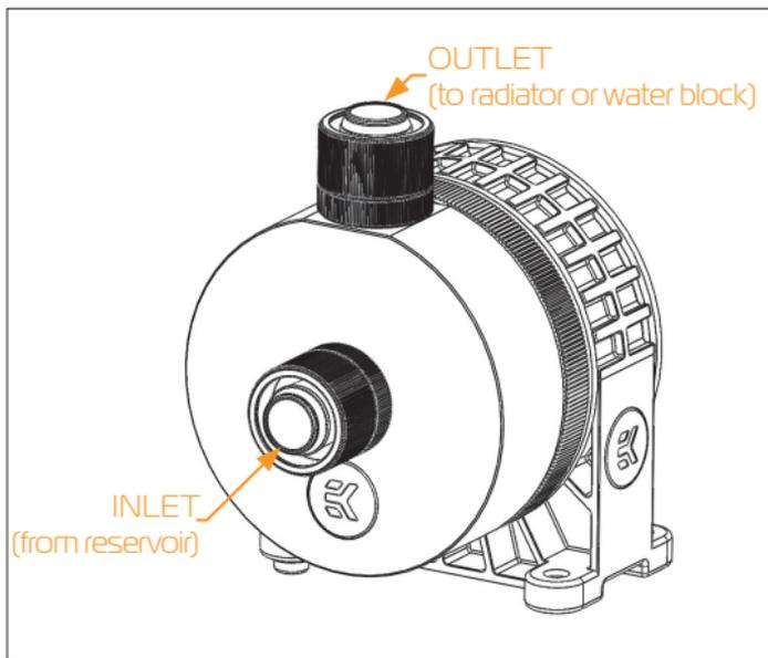
Screw in the fittings in the G1/4 threaded openings on plastic top. EKWB recommends using EK-ACF fittings with the EK-XTOP Revo D5 series pump tops. To ensure that the tubes are securely attached to the barb/fittings, please use hose clamps or an appropriate substitute.
