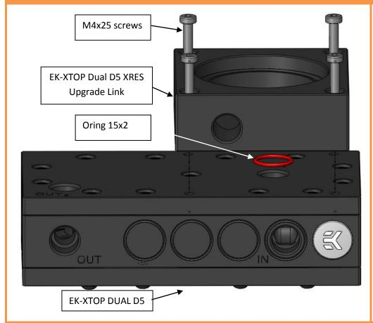
Make sure holes between Link and Top are concentric e.g. all ports are facing same direction. The orientation is very important in order to provide flow optimized by product design. In case of vortex occurance please use enclosed foam and make it fit into chamber.
