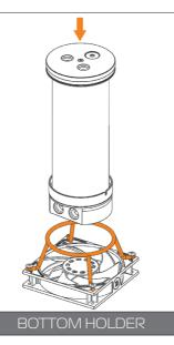
In RES X4 I2Umm fan holder should be mounted before this step. Take the reservoir and guide the bottom part through the circular part of the holder. The holder has a seat on the bottom manifold of the RES X4. Make sure that holder grabs the whole circumference of the reservoir bottom firmly.
