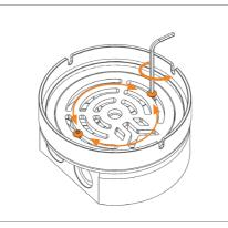
Unscrew two (2) M3 screws with enclosed 2 Allen key holding anticyclon in order to install the enclosed EK-HD Tubes. You can also unscrew it and rotate a bit.
