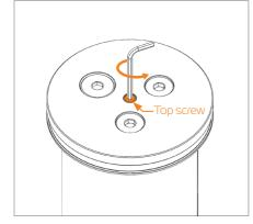
Unscrew the top screw with enclosed 2.5 Allen key and take the top of. Then remove the glass tube. You can also unscrew the center rod and anticyclon.
