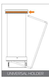
**STEP 1:** Take the RES X4 reservoir and guide the RES X4 Bottom into the bottom circular jaws of the holder.
