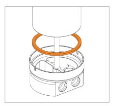
When reassembling the reservoir make sure the top and bottom gasket are in place. Put the glass tube on the bottom. Put the top gasket and top back on and screw the top screw.
