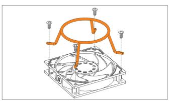
The RES X4 120mm fan holder is intended to be mounted on the bottom of the chassis . The gap between the mounting holes is 105mm, therefore it can also be mounted on 120mm fan holes. If you want to mount the holder on the fan, you should use 4 (four) self-tapping screw, otherwise you must use the enclosed 4 (four) M4x10 DIN 7984 screws, secured with nuts and washers.
