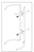
The RES X4 UNI holder is intended to be mounted anywhere in the chassis and in any possible direction. The gap between the mounting holes is 105mm, therefore it can also be mounted on 120mm fan holes. Secure the holder using the 2 (two) M4x10 DIN 7984 screws, PVC washers and M4 nuts.
