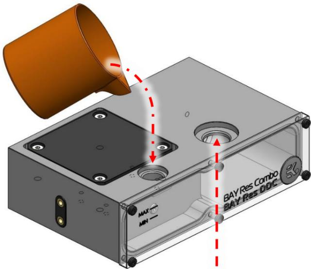
During this procedure G 3/8 threaded fill port must be opened.
