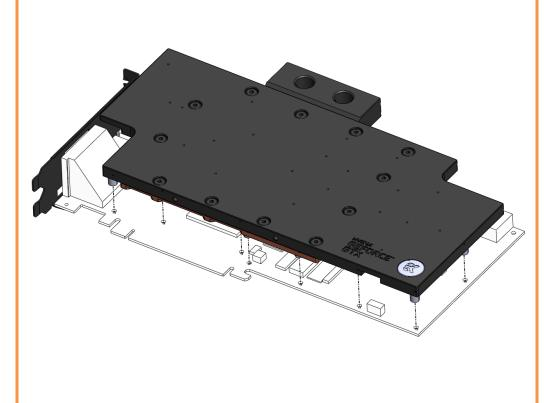
2. ATTACHING THE BLOCK TO THE GRAPHIC CARD. Use a Philips screwdriver screw with the enclosed M2,5x4 AX1 screws. EKWB recommends users to start tightening the screws around the GPU core and continue outwards. <u>Always use</u> a plastic washer under each and every screw! If the washer is already present on the circuit board (usually around the four GPU core screw holes) there is no need for additional washer. Enclosed M2x5 and M2 nut is for securing the I/O bracket as shown on picture below.
