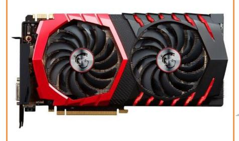
1. REMOVING STOCK COOLER: Remove all encircled screws using Phillips screwdriver. All heat sink assembly screws should be removed, including self-adhesive washers on both sides of the PCB (if present). After you remove the housing do not forget to unplug the fan and LED connector headers.
