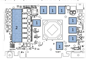
4. ATTACHING THE BLOCK TO THE GRAPHIC CARD: Use a Philips screwdriver screw with the enclosed M2,5x4 AX1 screws. EKWB recommends users to start tightening the screws around the GPU core and continue outwards. <u>Always use</u> a plastic washer under each and every screw! If the washer is already present on the circuit board (usually around the four GPU core screw holes) there is no need for additional washer.
