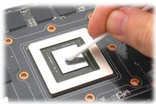
2. APPLYING THERMAL COMPOUND: Wipe off the remains (by using non-abrasive cloth or q-tip) of the original thermal compound until the components and circuit board are completely clean. Apply thermal compound: lightly coat NVIDIA GPU chip with enclosed EK-TIM Ectotherm thermal grease. EKWB recommends to apply thermal grease in cross form for best performance (see sample picture).
