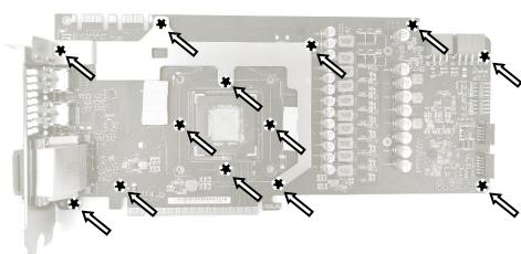
Remove two screws on the IO bracket using Phillips screwdriver
