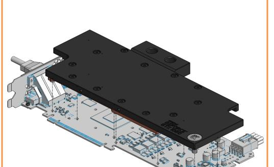
2. ATTACHING THE BLOCK TO THE GRAPHIC CARD. Use a Philips screwdriver screw with the enclosed M2,5x4 AX1 screws and one M2,5x6 AX1 screw. EKWB recommends users to start tightening the screws around the GPU core and continue outwards. <u>Always use</u> a plastic washer under each and every screw! If the washer is already present on the circuit board (usually around the four GPU core screw holes) there is no need for additional washer.
