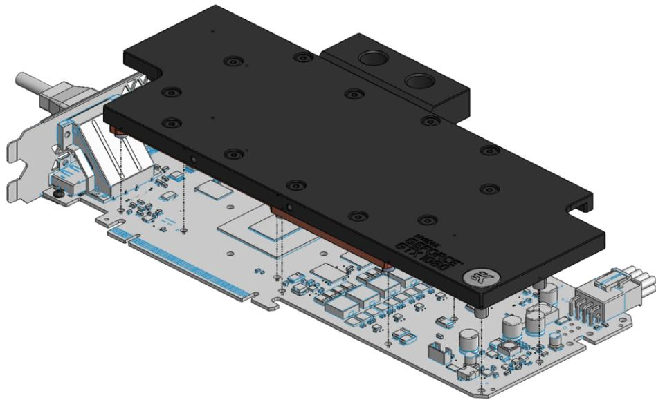
**2. ATTACHING THE BLOCK TO THE GRAPHIC CARD.** Use a Philips screwdriver screw with the enclosed M2,5x4 AX1 screws and one M2,5x6 AX1 screw. EKWB recommends users to start tightening the screws around the GPU core and continue outwards. **Always use** a plastic washer under each and every screw! If the washer is already present on the circuit board (usually around the four GPU core screw holes) there is no need for additional washer.
