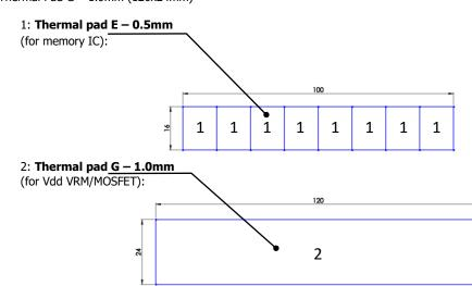
4. PLACING THERMAL PADS ON PCB. Place thermal pads on the circuit board as shown on the picture below. Refer to numbering in previous picture when applying thermal pads of different sizes or thicknesses. EK made sure to provide customers with more than adequate quantity of thermal pads to complete this step.
