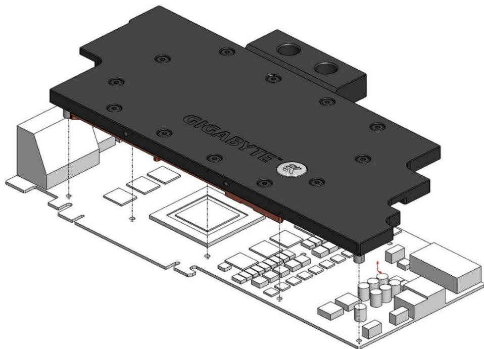
**2. ATTACHING THE BLOCK TO THE GRAPHIC CARD.** Use a Philips screwdriver screw with the enclosed M2,5x4 DIN 7985 screws. EKWB recommends users to start tightening the screws around the GPU core and continue outwards. Always use a plastic washer under each and every screw! If the washer is already present on the circuit board (usually around the four GPU core screw holes) there is no need for additional washer.
