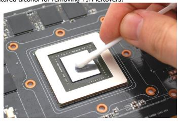
3. APPLYING THERMAL COMPOUND: Wipe off the remains (by using non–abrasive cloth or *q-tip*) of the original thermal compound until the components and circuit board are completely clean. Apply thermal compound: lightly coat *AMD* GPU chip with enclosed EK-TIM Ectotherm thermal grease. EKWB recommends to apply thermal grease in cross form for best performance (see sample picture).
