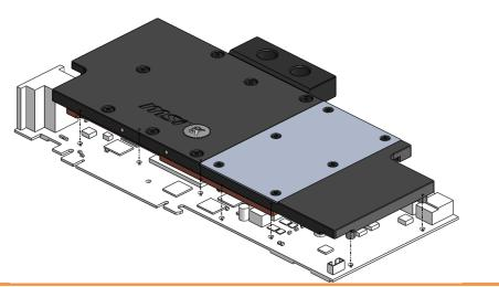
3. ATTACHING THE BLOCK TO THE GRAPHIC CARD: Use a Philips screwdriver with the enclosed M2.5x4 DIN 7985 screws with PVC washers. EKWB recommends users to start tightening the screws around the GPU core and continue outwards.
