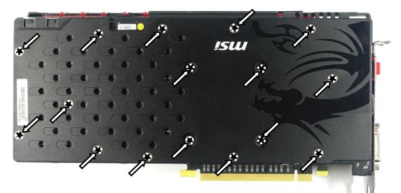
2. CLEANING THE PCB: Carefully detach the original stock cooler after removing **all** screws securing it to the board. Wipe off the remains (by using non–abrasive cloth or *qtip*, as shown on sample photo) of the original thermal compound until the components and circuit board are completely clean. EKWB recommends the use of denatured alcohol for removing TIM leftovers.
