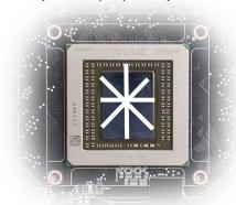
4. CUTTING THERMAL PADS: Your block comes with thermal pads. Some of the pads have to be cut to smaller chunks in order to cover all the memory, VRM components such as MOSFETs and drivers. PLEASE REMOVE THE PROTECTIVE FOIL FROM BOTH SIDES OF THE THERMAL PADS PRIOR TO INSTALLATION.
