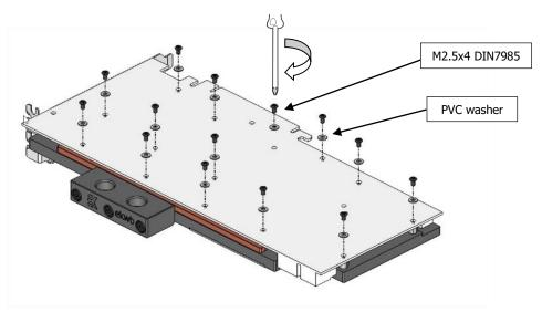
3. (OPTIONAL) ATTACHING THE BLOCK AND THE MSI BACKPLATE TO THE GRAPHIC CARD: Use a Philips screwdriver with the enclosed 4 (four) M2.5x4 DIN 7985 screws around GPU core and 10 (ten) M2.5x6 DIN 7985 screws for the MSI backplate. Please apply the PVC washers only with four screws around the GPU core. EKWB recommends users to start tightening the screws around the GPU core and continue outwards.
