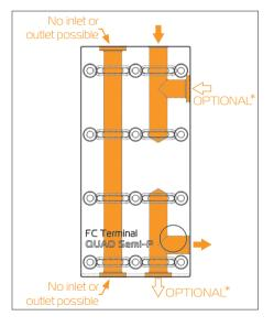
\* Every optional hole can be used with EK-Extender GI/4 – Nickel EAN: 3831109845165
