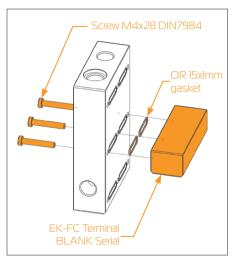
Tighten the three (3) enclosed M4x28 DIN7984 screws to EKFC Terminal BLANK Serial using Allen (hex) key 2.5mm.
